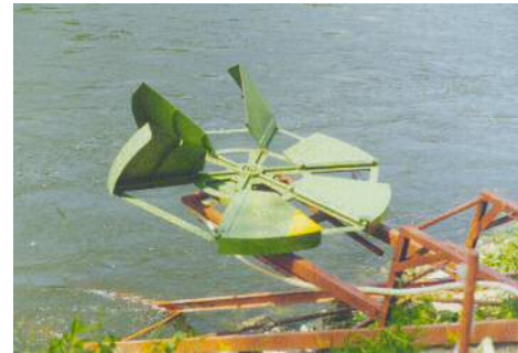
Left: smallest SP1 turbine with diameter of 0,9 m on lifting ramp.
