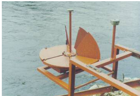
Left: smallest SP1 turbine with diameter of 0,9 m on lifting ramp.
